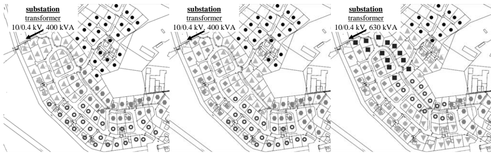
(a) design value of 3.0 kVA per household (b) design value of 3.5 kVA per household (c) design value of 5.9 kVA per household
